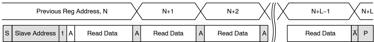
Figure 38. Single READ from Current Location
