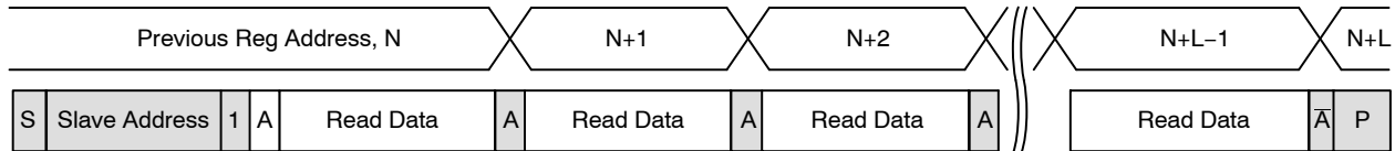
Figure 40. Sequential READ, Start from Current Location
