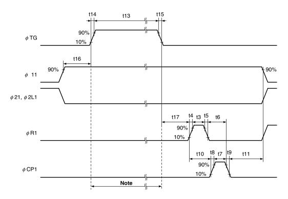
**Note** Set the  $\phi$  R and  $\phi$  CP to low level during this period.
