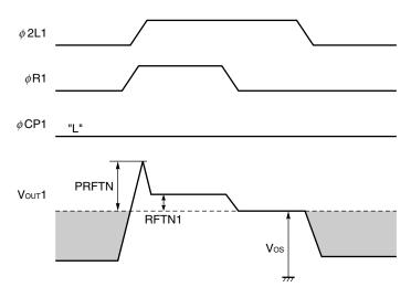
Caution This shows timing of Vout1 side ( $\phi$ 2L1,  $\phi$ R1,  $\phi$ CP1, Vout1). The definition of Vout2 side ( $\phi$ 2L2,  $\phi$ R2,  $\phi$ CP2, Vout2) is equal.
