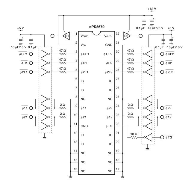
Cautions 1. Leave pins 6, 7, 12, 13, 20, 21, 26 and 27 (IC) unconnected.2. Connect the No connection pins (NC) to GND.
