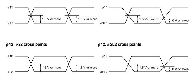
**Remark** Adjust cross points of ( $\phi$  11,  $\phi$  21), ( $\phi$  11,  $\phi$  2L1), ( $\phi$  12,  $\phi$  22) and ( $\phi$  12,  $\phi$  2L2) with input resistance of each pin.
