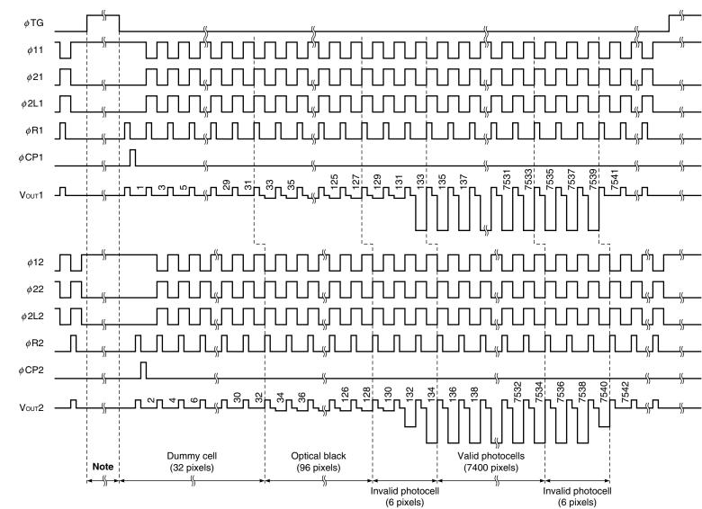
**Note** Set the  $\phi$  R1,  $\phi$  R2,  $\phi$  CP1 and  $\phi$  CP2 to low level during this period.
