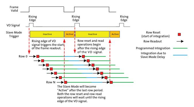
The row shutter and read operations will stop when the slave mode becomes active and is waiting for the VD signal. The following should be considered when configuring the sensor to use the slave mode:
