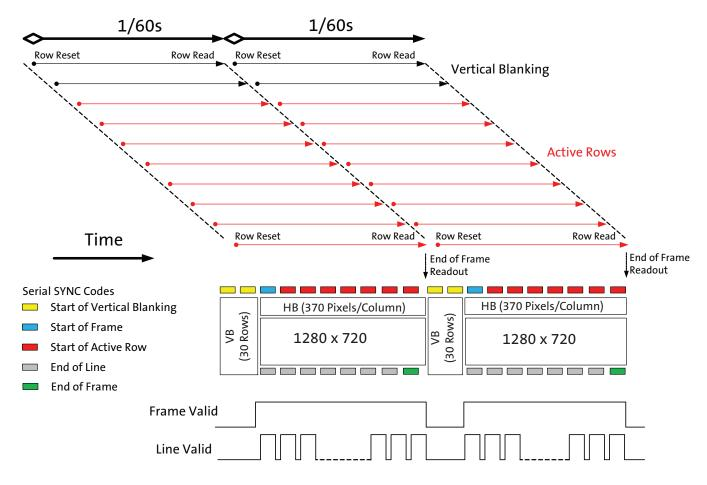
Figure 29 aligns the frame integration and readout operation to the sensor output. It also shows the sensor output using the HiSPi Streaming-SP protocol. Different sensor protocols will list different SYNC codes.
