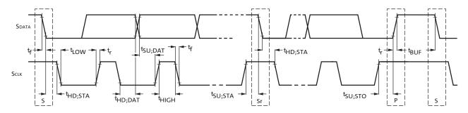
Note: Read sequence: For an 8-bit READ, read waveforms start after WRITE command and register address are issued.
