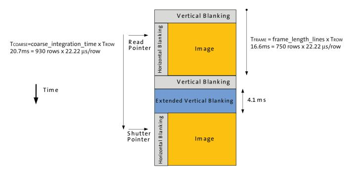
The minimum frame-time is defined by the number of row periods per frame and the row period. The sensor frame-time will increase if the *coarse\_integration\_time* is set to a value equal to or greater than the *frame\_length\_lines*.
