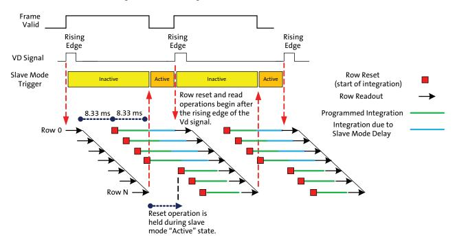
When the slave mode becomes active, the sensor will pause both row read and row reset operations. (Note: The row integration period is defined as the period from row reset to row read.) The frame-time should therefore be configured so that the slave mode "wait period" is as short as possible. In the case where the sensor integration time is shorter than the frame time, the "wait period" will only increase the integration of the rows that have been reset following the last VD pulse.
