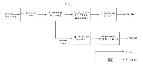
The sensor will use op\_sys\_clk\_div and op\_pix\_clk\_div to configure the output clock per lane (CLK\_OP). The configuration will depend on the number of active lanes (1, 2, or 4) configured.
