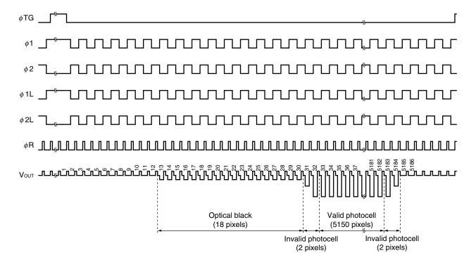
Caution Input the  $\phi$ R pulse continuously during the high level period of  $\phi$ TG.
