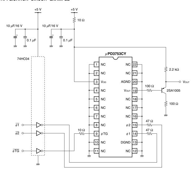
Caution Connect the No connection pins (NC) to GND.
