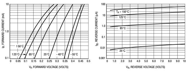
Figure 2. Typical Forward Voltage
