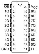
A buffered output-enable ( $\overline{OE}$ ) input can be used to place the eight outputs in either a normal logic state (high or low) or the high-impedance state. In the high-impedance state, the outputs neither load nor drive the bus lines significantly. The high-impedance state and increased drive provide the capability to drive bus lines without interface or pullup components.
