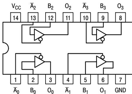
Figure 1. Pinout: 14-Lead Packages Conductors (Top View)
