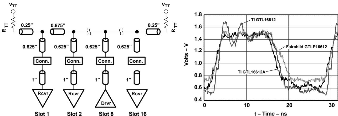
**Figure 1. Test Backplane Model With Output Waveform Results**
