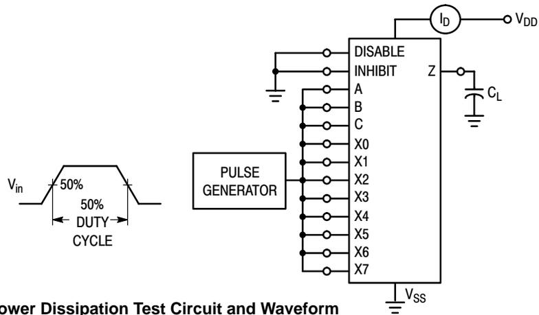
Figure 1. Power Dissipation Test Circuit and Waveform
