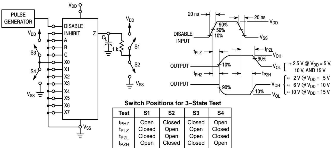
Figure 3. 3-State AC Test Circuit and Waveform
