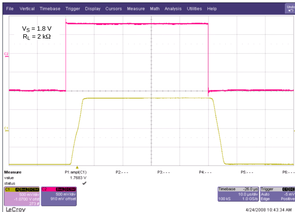
Figure 18. Small Signal Noninverting Response
