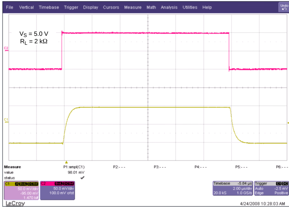
Figure 18. Small Signal Noninverting Response
