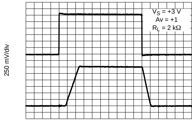
Figure 24. 3 V Non-Inverting Large Signal Pulse Response
