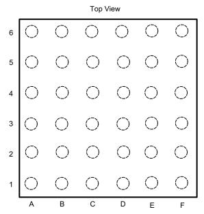
Figure 2. Top View (Bump Side Down)
