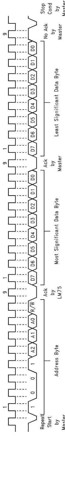
(c) Typical 1-Byte Read From Configuration Register With Preset Pointer
