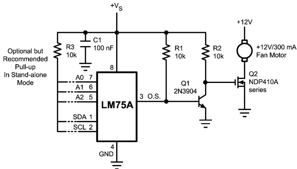
When using the two-wire interface: program O.S. for active high and connect O.S. directly to Q2's gate.
