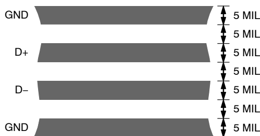
Figure 22. Typical Arrangement of Signal Tracks
