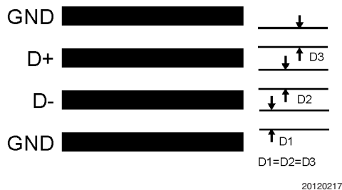
FIGURE 4. Ideal Diode Trace Layout
