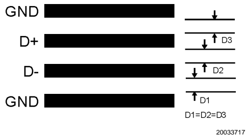
FIGURE 15. Ideal Diode Trace Layout
