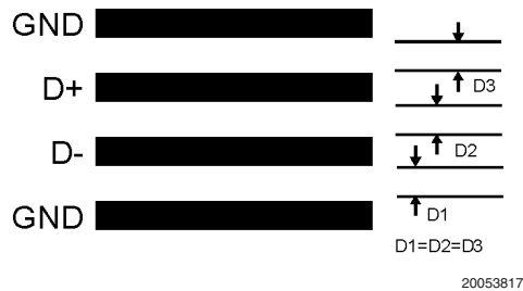
FIGURE 11. Ideal Diode Trace Layout
