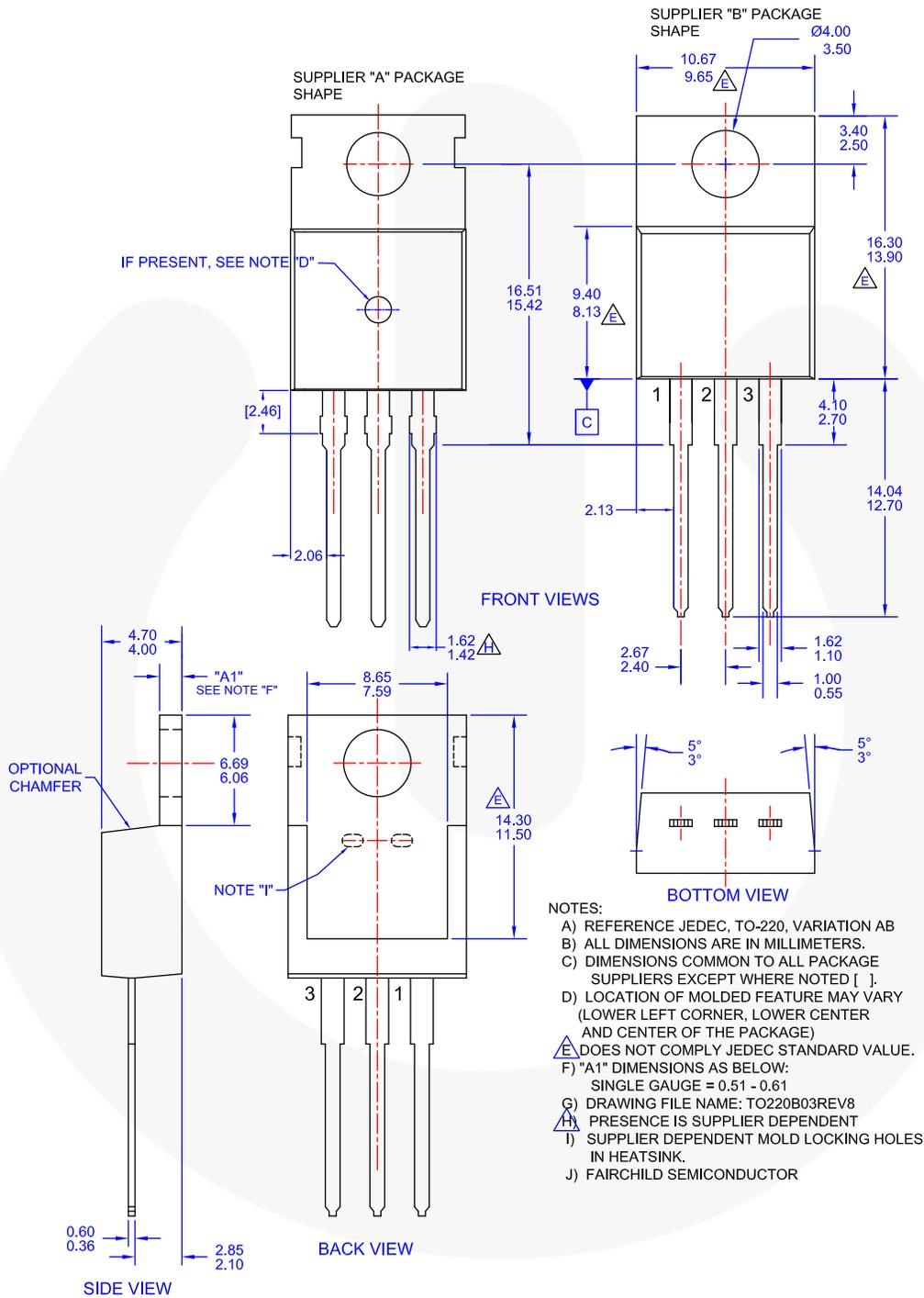
Figure 6. TO-220, MOLDED, 3LEAD, JEDEC VARIATION AB
