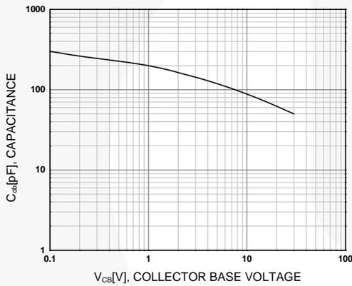
Figure 3. Collector Capacitance
