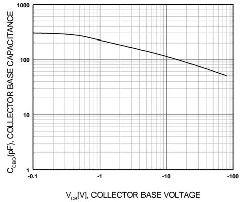
Figure 4. Collector-Base Capacitance
