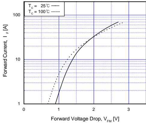
Fig 18. Forward Characteristics
