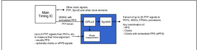
FIGURE 2-1: TimeBuffer Application Example.
