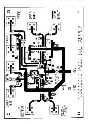
Figure 29. Positive Supply Configuration: Component Side (Top Layer)
