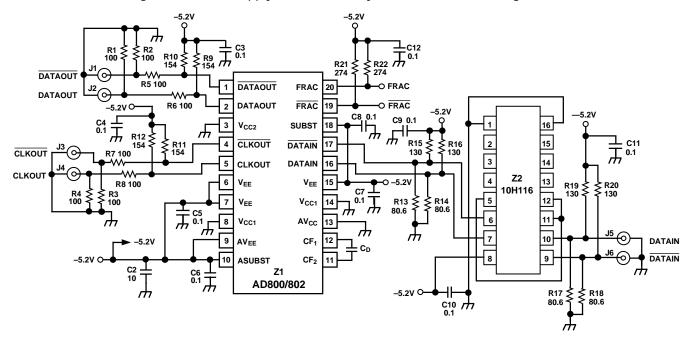
Figure 26. Evaluation Board Schematic, Negative Supply
