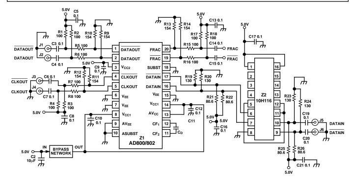
Figure 22. Evaluation Board Schematic, Positive Supply
