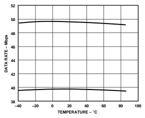
Figure 5. AD800-45 Capture and Tracking Range vs. Temperature
