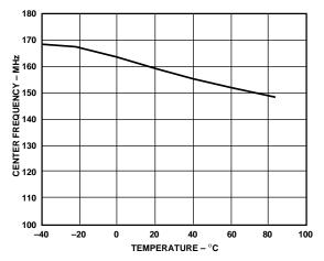
Figure 15. AD802-155 Center Frequency vs. Temperature
