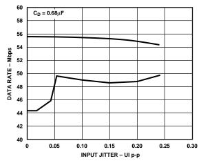
Figure 13. AD800-52 Acquisition Range vs. Input Jitter
