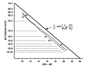
Figure 14. AD800-52 Bit Error Rate vs. Input Jitter
