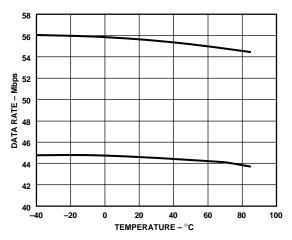
Figure 11. AD800-52 Capture and Tracking Range vs. Temperature
