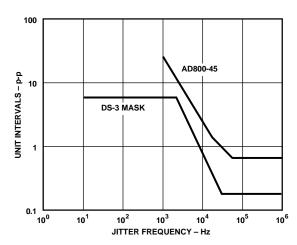
Figure 6. AD800-45 Jitter Tolerance
