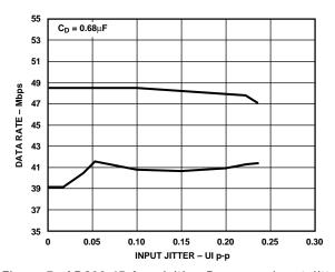
Figure 7. AD800-45 Acquisition Range vs. Input Jitter
