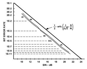
Figure 8. AD800-45 Bit Error Rate vs. Input Jitter
