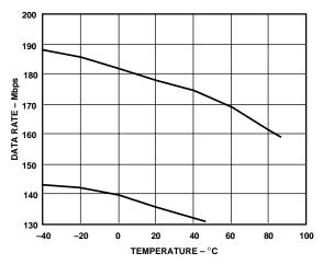
Figure 17. AD802-155 Capture Range, Tracking Range vs. Temperature
