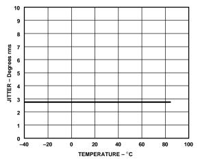
Figure 10. AD800-52 Jitter vs. Temperature
