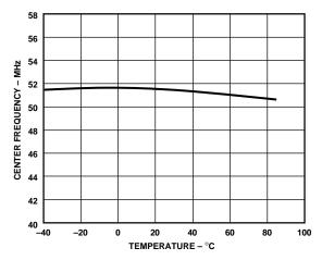
Figure 9. AD800-52 Center Frequency vs. Temperature
