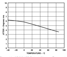
Figure 16. AD802-155 Output Jitter vs. Temperature
