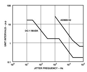
Figure 12. AD800-52 Jitter Tolerance
