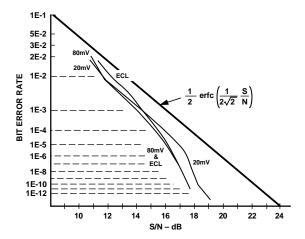
Figure 20. AD802-155 Bit Error Rate vs. Input Jitter
