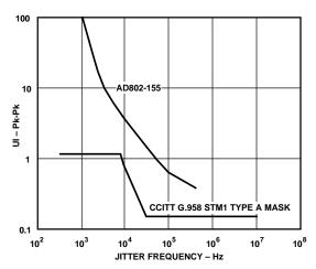
Figure 18. AD802-155 Jitter Tolerance
