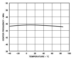
Figure 3. AD800-45 Center Frequency vs. Temperature
