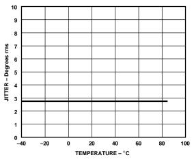
Figure 4. AD800-45 Jitter vs. Temperature
