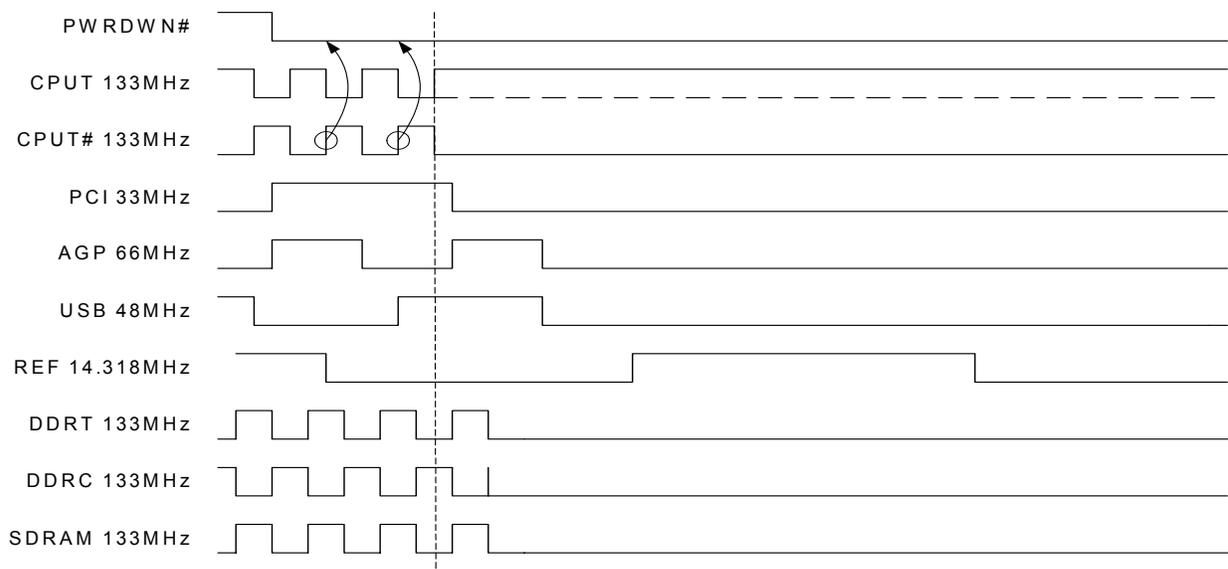
**Figure 2. Power-down Assertion Timing Waveform (in P4 mode)**
