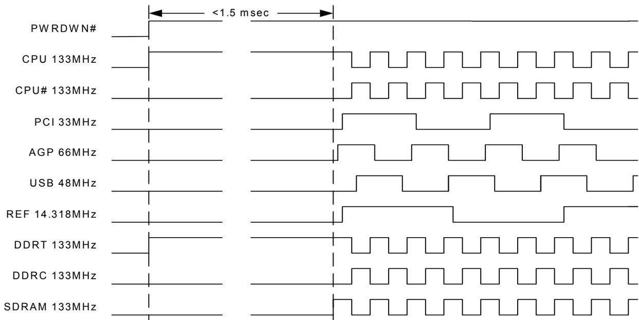
**Figure 3. Power-down Deassertion Timing Waveform (in P4 mode)**
