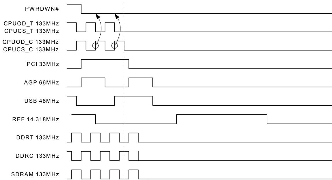
**Figure 4. Power-down Assertion Timing Waveform (in K7 mode)**
