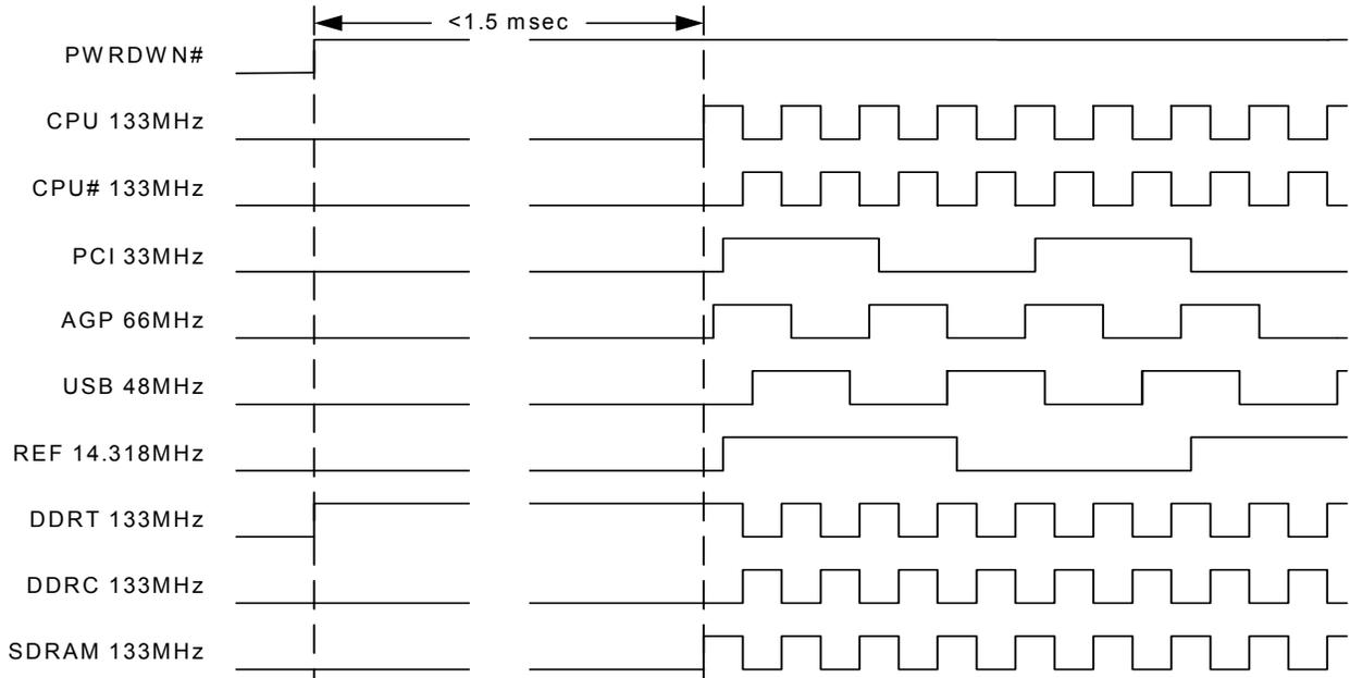
**Figure 5. Power-down Deassertion Timing Waveform (in K7 Mode)**
