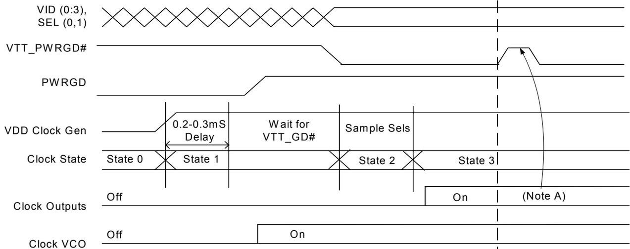
**Figure 6. VTT\_PWGD# Timing Diagram (With Advanced PLL Processor SelP4\_K7 = 1)<sup>[3]</sup>**
