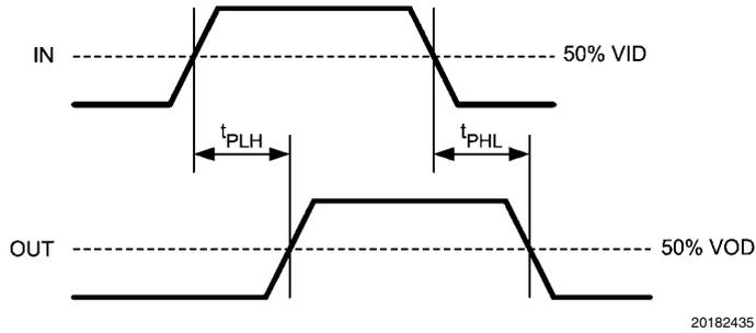
FIGURE 3. Propagation Delay
