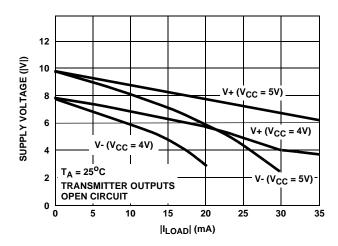
FIGURE 6. V+, V- OUTPUT VOLTAGE vs LOAD
