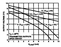
FIGURE 2. V+, V- OUTPUT VOLTAGES vs LOAD CURRENT
