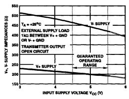
FIGURE 1. V+, V- OUTPUT IMPEDANCES VS VCC
