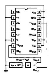
FIGURE 9. POWER-OFF SOURCE RESISTANCE CONFIGURATION
