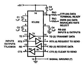
FIGURE 10. SIMPLE DUPLEX RS-232 PORT WITH CTS/RTS HANDSHAKING
