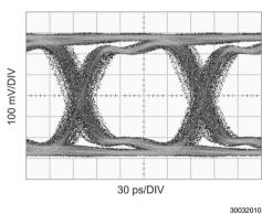
Figure 10. Equalized Signal (40 In FR4, 6.4 Gbps, PRBS7, 0x06 Setting)
