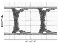
Figure 8. Equalized Signal (40 In FR4, 2.5Gbps, PRBS7, 0x07 Setting)
