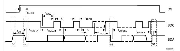
FIGURE 7. SMBus Timing Parameters
