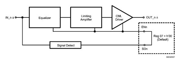
**FIGURE 9. Automatic Enable Configuration**
