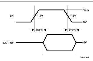
FIGURE 5. Enable (EN) Delay Timing Diagram
