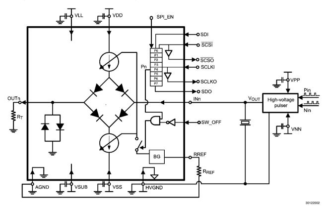
FIGURE 3. Block Diagram of T/R Channel
