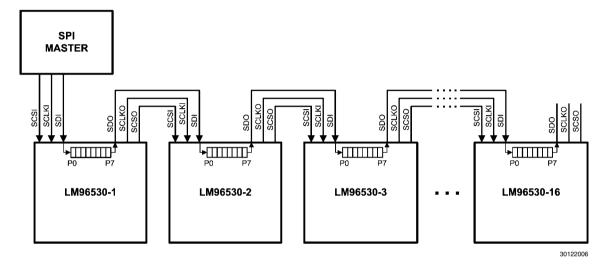
FIGURE 4. 16 LM96530 Devices Daisy Chained @ SCLKI = 16MHz
