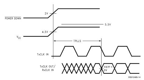
FIGURE 11. DS90CF561 (Transmitter) Phase Lock Loop Set Time
