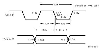
FIGURE 7. DS90CF561 (Transmitter) Setup/Hold and High/Low Times
