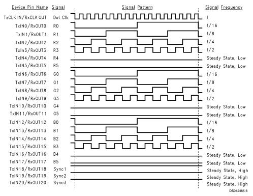
FIGURE 2. "16 Grayscale" Test Pattern (Notes 7, 8, 9, 10)
