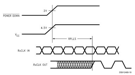
FIGURE 12. DS90CF562 (Receiver) Phase Lock Loop Set Time
