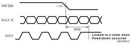
FIGURE 16. Receiver Powerdown Delay
