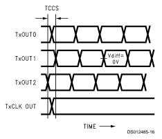
Measurements at Vdiff = 0V TCCS measured between earliest and latest initial LVDS edges. TxCLK OUT Differential High→Low Edge for DS90CF561
