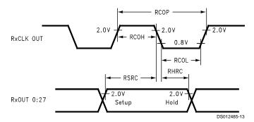
FIGURE 8. DS90CF562 (Receiver) Setup/Hold and High/Low Times
