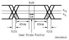
SW — Setup and Hold Time (Internal Data Sampling Window)
