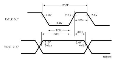
FIGURE 3. DS90CR286A/DS90CR216A (Receiver) Setup/Hold and High/Low Times
