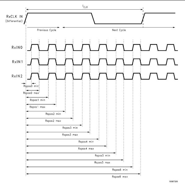
FIGURE 10. DS90CR216A (Receiver) LVDS Input Strobe Position
