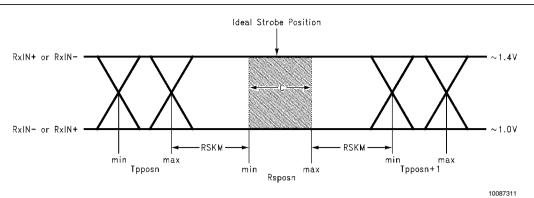
C—Setup and Hold Time (Internal data sampling window) defined by Rspos (receiver input strobe position) min and max
