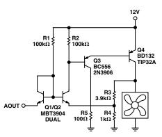
Figure 9f. Discrete Fan Drive Circuit with Bipolar Output Dual Supply
