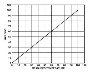
TPC 4. ADM1024 Reading vs. Pentium® III Temperature Measurement
