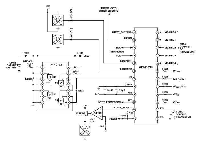
Figure 18. Application Circuit
