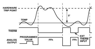
Figure 16b. THERM Output in ACPI Mode
