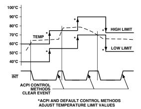
Figure 15. Operation of INT for Temperature Interrupts
