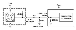
Figure 10d. Fan with Strong Tach. Pull-Up to  $>V_{CC}$  or Totem-Pole Output, Attenuated with R1/R2
