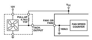
Figure 10a. Fan with Tach. Pull-Up to  $+V_{CC}$
