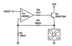
*Figure 9a. Fan Drive Circuit with Op Amp and Emitter-Follower*
