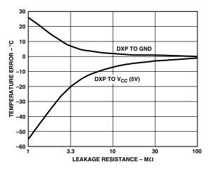
TPC 1. Temperature Error vs. PC Board Track Resistance
