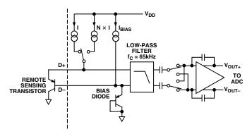
Figure 7. Signal Conditioning for External Diode Temperature Sensors
