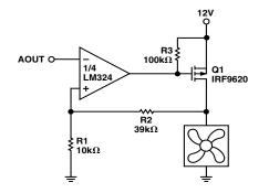
Figure 9c. Fan Driver Circuit with Op Amp and P-Channel MOSFET
