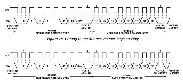
Figure 2c. Reading Data from a Previously Selected Register
