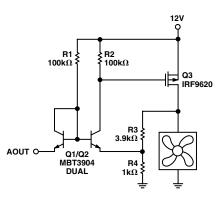
Figure 9d. Discrete Fan Drive Circuit with P-Channel MOSFET, Single Supply
