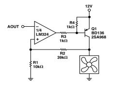
*Figure 9b. Fan Drive Circuit with Op Amp and PNP Transistor*
