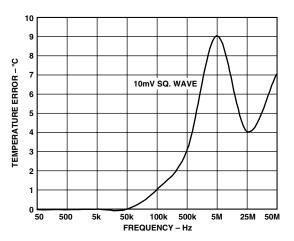
TPC 6. Temperature Error vs. Differential-Mode Noise Frequency
