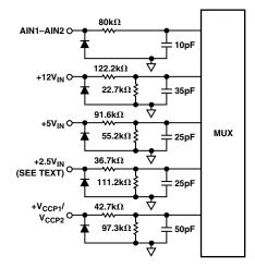
Figure 3. Structure of Analog Inputs
