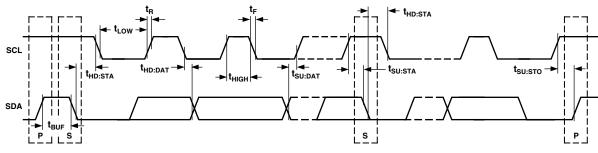
Figure 1. Diagram for Serial Bus Timing
