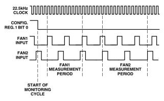
Figure 11. Fan Speed Measurement
