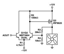
Figure 9e. Discrete Fan Drive Circuit with P-Channel MOSFET, Dual Supply
