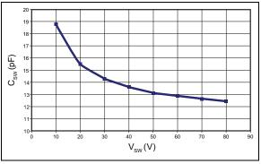
FIGURE 3-1: C<sub>TX-RX</sub> vs. V<sub>TX-RX</sub>.
