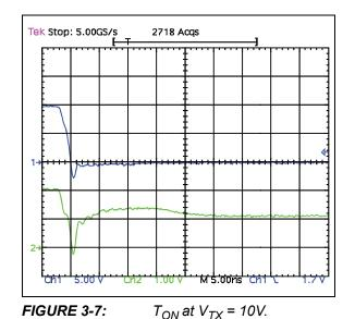
Figure 3-7 illustrates the actual waveform and measurement of the  $T_{ON}$ . The  $T_{ON}$  is measured from 2V of the  $V_{TX}$  to 1V of the  $V_{RX}$ .
