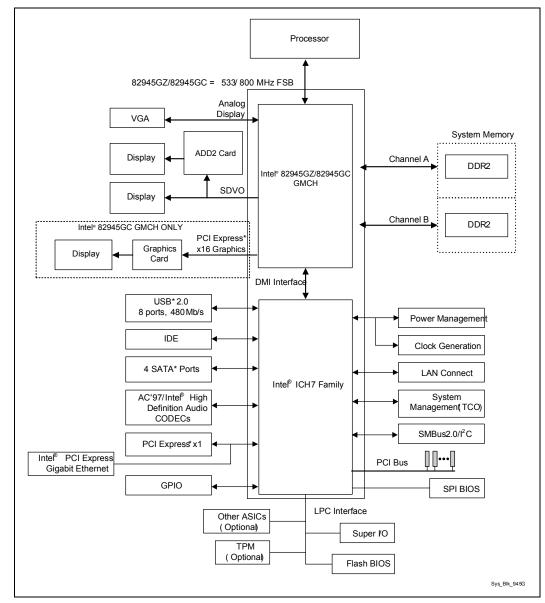
Figure 1-2. Intel<sup>®</sup> 945GZ/82945GC Express Chipset System Block Diagram Example
