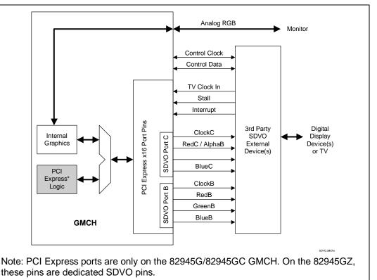
Figure 10-2. SDVO Conceptual Block Diagram
