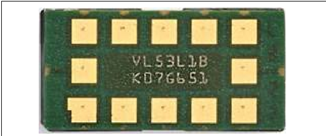
Figure 22. Example of prototype marking
