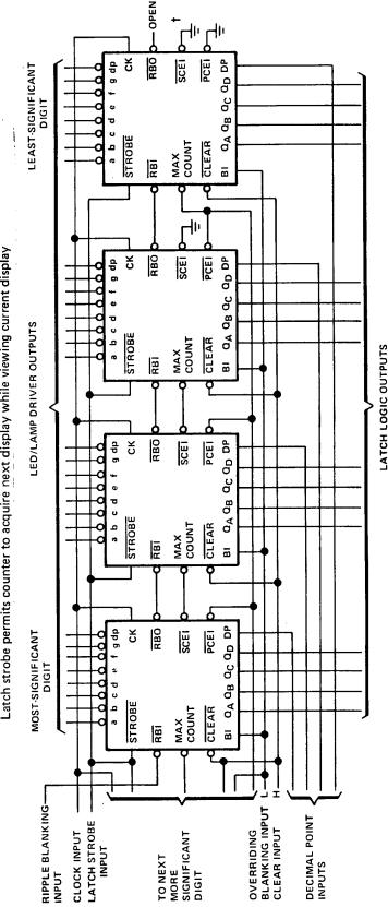
entire counter (high to disable, low to count) provided the logic level on this pin is not changed while the clock line is low or false counting †The serial count-enable input of the least-significant digit is normally grounded; however, it may be used as a count-enable control for the may result.
