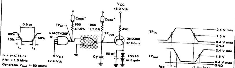
$C_T = 15 \text{ pF}$  = total parasitic capacitance, which includes probe, wiring, and load capacitances.
