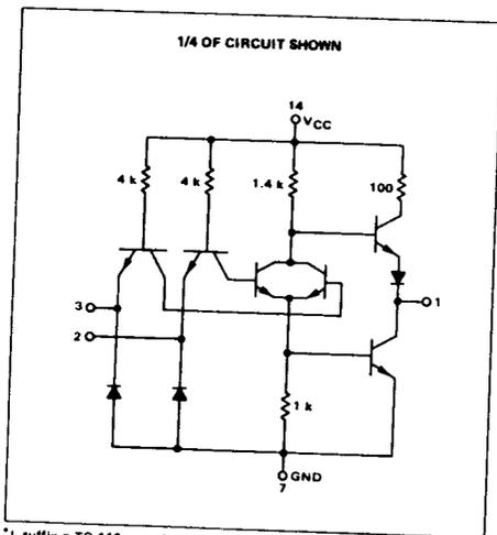
This device consists of four 2-input NOR gates. Each gate may be used as an inverter, or two gates may be cross-coupled to form bistable circuits.
