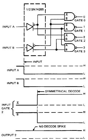
FIGURE D - SYMMETRICAL DECODER/CODE CONVERTER
