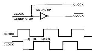
FIGURE A - TYPICAL CLOCK/CLOCK GENERATOR CIRCUIT
