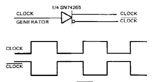
FIGURE B - SKEWLESS CLOCK/CLOCK GENERATOR CIRCUIT
