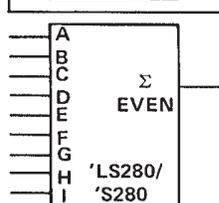
As an alternative, the outputs of two or three parity generators/checkers can be decoded with a 2-input ('S86 or 'LS86) or 3-input ('S135) exclusive-OR gate for 18- or 27-line parity applications.
