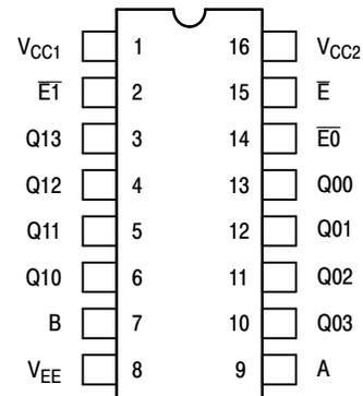
Pin assignment is for Dual-in-Line Package.
