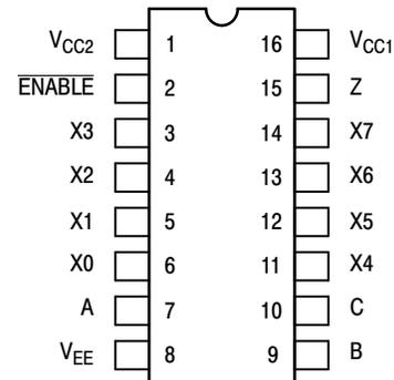
Pin assignment is for Dual-in-Line Package.
