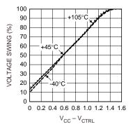
Typical Voltage Output Swing V<sub>CC</sub> = 3.3V or 5V
