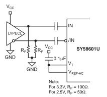
Figure 3d. LVPECL Interface (AC-Coupled)
