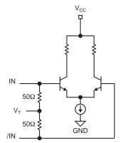
Figure 2a. Simplified Differential Input Stage
