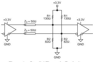
Figure 4a. Parallel Thevenin-Equivalent Termination
