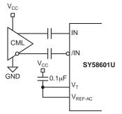
Figure 3b. CML Interface (AC-Coupled)
