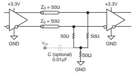
Figure 4b. Parallel Termination (3-Resistor)
