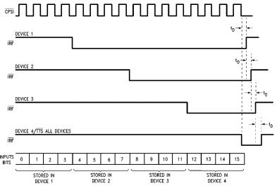
FIGURE 7. Serial Data Entry for Array of Figure 6
