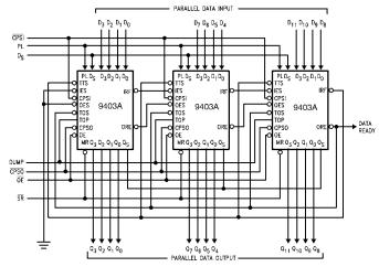
FIGURE 5. A Horizontal Expansion Scheme
