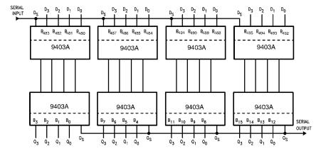
FIGURE 9. Final Position of a 496-Bit Serial Input
