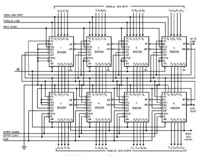
FIGURE 6. A 31x16 FIFO Array
