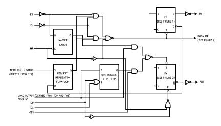
FIGURE 10. Conceptual Diagram, Interlocking Circuitry
