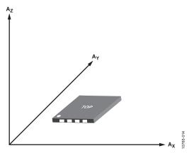
Figure 14. Axes of Acceleration Sensitivity (Corresponding Output Voltage Increases When Accelerated Along the Sensitive Axis)
