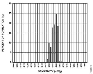
Figure 10. Y-Axis Sensitivity at 25°C,  $V_S = 3 V$
