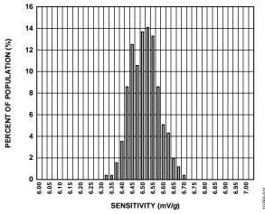
Figure 11. Z-Axis Sensitivity at 25°C,  $V_S = 3 V$
