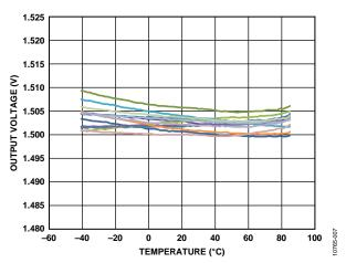
Figure 7. Y-Axis Zero g Offset vs. Temperature,  $V_S = 3 V$  (14 Parts Soldered to PCB)
