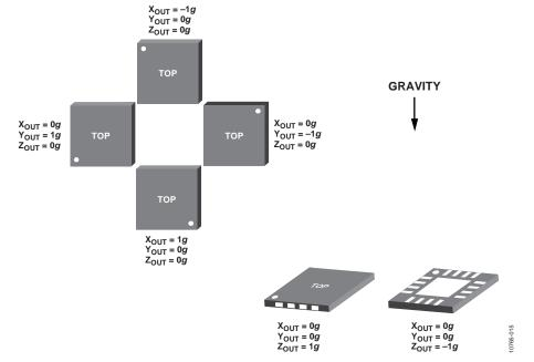
Figure 15. Output Response vs. Orientation to Gravity
