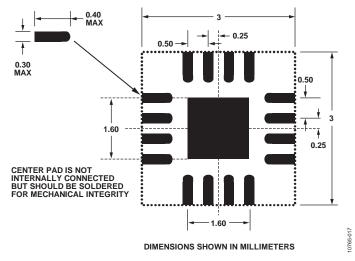
Figure 17. Recommended PCB Layout
