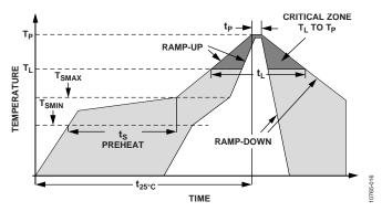
Figure 16. Recommended Soldering Profile
