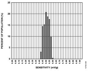
Figure 9. X-Axis Sensitivity at 25°C,  $V_S = 3 V$
