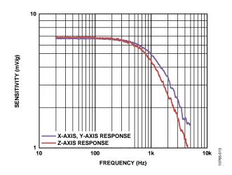
Figure 13. Typical Frequency Response
