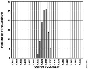
Figure 4. Y-Axis Zero g Output Voltage at 25°C,  $V_S = 3 V$
