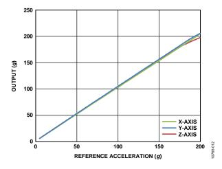
Figure 12. Typical Output Linearity over the Dynamic Range
