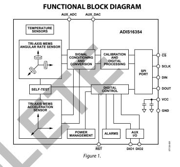
compensates for all major influences on the MEMS sensors, thus maintaining highly accurate sensor outputs without further testing, circuitry, or user intervention.
