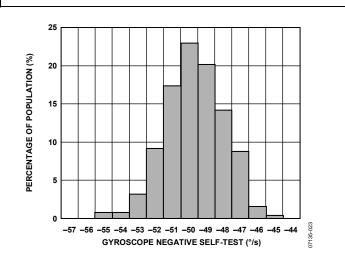
Figure 24. Gyroscope Negative Self-Test Distribution, 25°C
