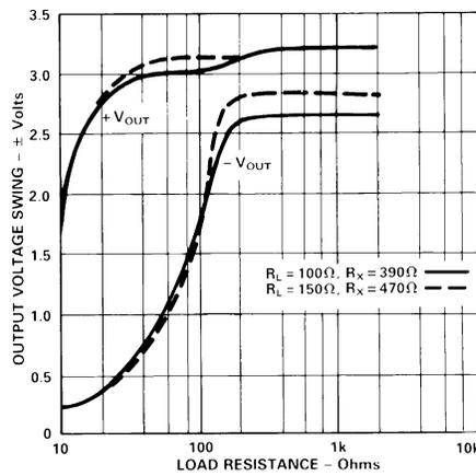
Figure 2. Output Voltage Swing vs. Load Resistance
