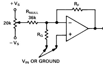
$$\text{OUTPUT NULL RANGE} \cong +V_s \left( \frac{R_F}{R_{NULL}} \right) \text{ TO } -V_s \left( \frac{R_F}{R_{NULL}} \right)$$
