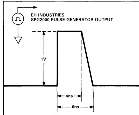
Figure 43. A Simulated Ideal Test Circuit Error Signal
