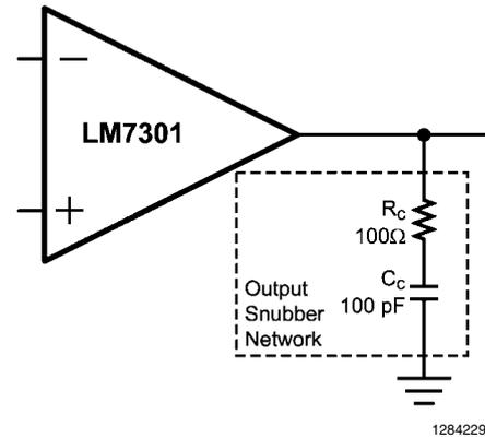
**FIGURE 8. Non-dissipating Snubber Network to Reduce Gain Peaking**
