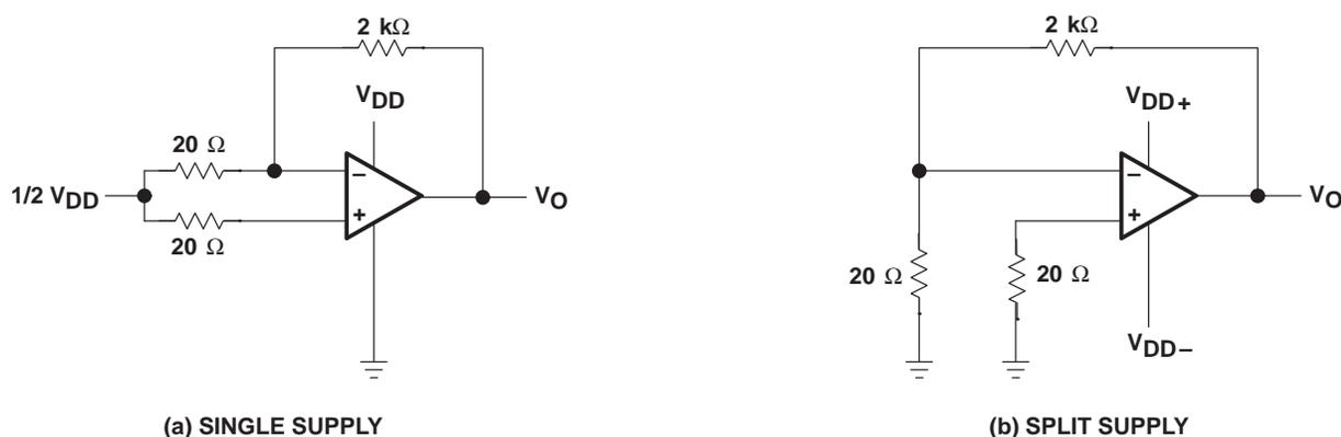
Figure 35. Noise-Test Circuit
