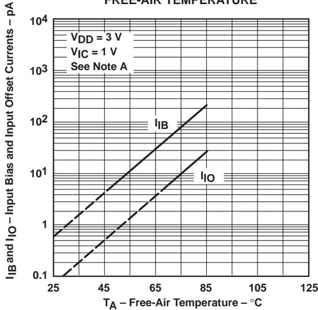
NOTE: The typical values of input bias current and input offset current below 5 pA were determined mathematically.
